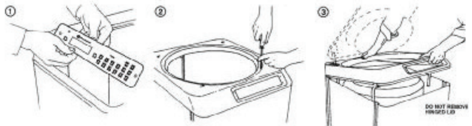
Figure 14. Removing the Cabinet Top of the 10K or 24K
