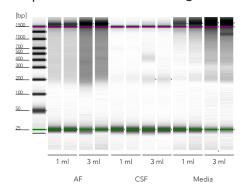
Amniotic fluid (AF), cerebrospinal fluid (CSF), or spent HeLa cell culture media (Media) were used to isolate cell-free nucleic acids using *Quick*-cfDNA/RNA<sup>™</sup> Serum & Plasma Kit. Endogenous cell-free DNA from each sample type was visualized using the Agilent 2200 Tapestation® system.
