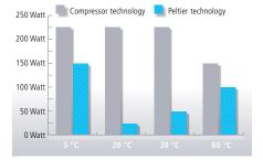
Up to 90 % less energy consumption at 22  $^{\circ}\mathrm{C}$  ambient temperature
