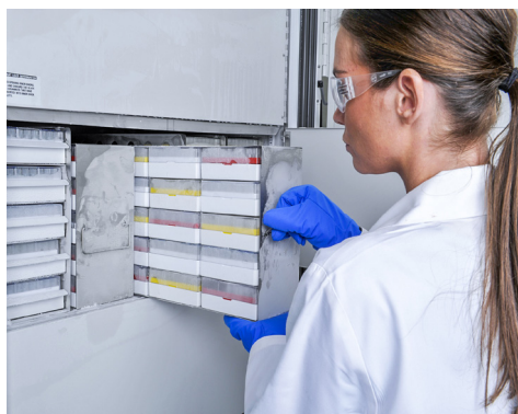
Side access racks
