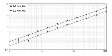
**FIGURE 1:** dsDNA quantitation on the SpectraDrop micro volume microplate. The ABS Plus reader with the SpectraDrop microplate could detect down to 2 and 4 ng/ $\mu$ l of DNA using the 1.0mm (blue) and 0.5mm (red) coverslips respectively.
