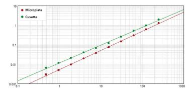
FIGURE 4: dsDNA quantitation in a 96-well microplate or cuvette. The dsDNA dilution series was detectable from 250 to 0,50ng/µl in both cuvette and microplate formats. Additionally, both dilution series demonstrated high linearity.
