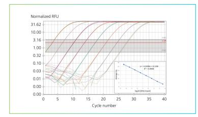
FIGURE 2: Samples from multiple NGS libraries were pooled into a test sample with average fragment size of 450bp. A 10-fold dilution series was prepared and assayed on the Q. Analysis of the resulting amplification curves showed high efficiency and sensitivity across an 8 log dynamic range.
