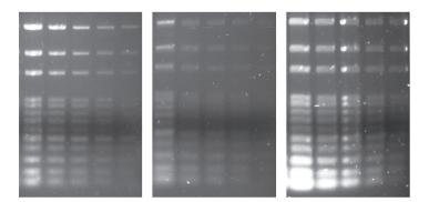
Comparison of EZ-Vision<sup>®</sup> Blue Light DNA Dye to GelGreen<sup>™</sup> and SYBR<sup>®</sup> Green I Two-fold dilution series of identical DNA fragments were electrophoresed in 1% agarose gels. The gels were then stained with EZ-Vision Blue Light (left panel), GelGreen (middle panel) and SYBR Green I (right panel). DNA fragments were visualized using a blue light transilluminator and SYBR Green filter.
