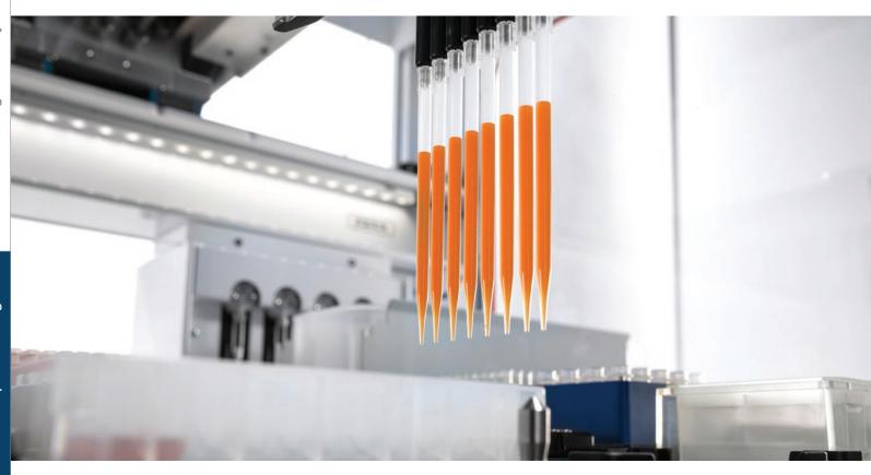
Conductive tips for use with Biomek Span-8 Pod to enable Liquid Level Sensing
