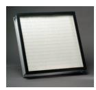
**82010-686\***—Replacement HEPA Filter. 99.99% efficient on particles 0.3 micron in size. Not suitable for use with biohazardous materials or volatile organic material. For use with FilterMate Portable Exhausters. Shipping weight 35 lbs.
