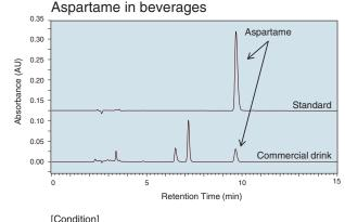
Column : LaChrom C18 (5 µm) 4.6 mm I.D.×250 mm L. Mobile phase : acetonitrile / (0.01 mol/L KH<sub>2</sub>PO<sub>4</sub> (pH = 3.18) = 15 : 85 Column temperature :  $40^{\circ}$ C Flow rate : 1.0 mL/min Detection : UV 210 nm Injection vol. : 10 µL (100 µg/mL)
