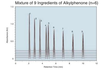
$$\label{eq:condition} \begin{split} & [Condition] \\ & Column: HITACHI LaChrom C18 (5 \ \mum) \ 4.6 \ mm \ I.D.x150 \ mm \ L. \\ & Mobile \ phase: A: CH_3CN \ B: H_2O \\ & Gradient \ program: 0 - 11 \ mm \ A \ 65 \ \rightarrow \ 100\% \\ & Column \ Temperature: 40^{\circ}C \\ & Flow \ rate: 1.0 \ mL/min \\ & Detection: UV \ 247 \ nm \\ & Injection \ vol.: 10 \ \muL \ (100 \ g/mL \ each.) \end{split}$$
