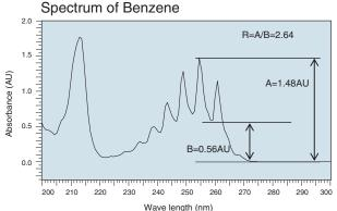
The 1,024-bit photo diode array is very effective for the measurement of samples such as Benzene, which has a characteristic UV spectrum.
