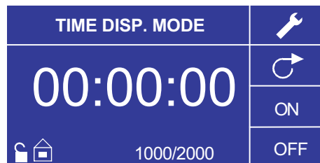
Figure 3-5. Time Dispense Mode Operation
