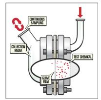
Permeation data is presented in two ways: Breakthrough time and Color code. Breakthrough times (min.) are the times observed from the start of the test to first detection of the chemical on the other side of the sample (see test chamber setup). These times represent how long a glove can be expected to provide effective permeation resistance when totally immersed in the test chemical.
